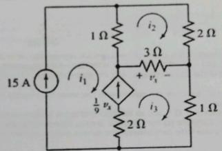
Q.2(a) Apply current division and resistance combination methods to find  $i_1$  and  $i_2$ .
