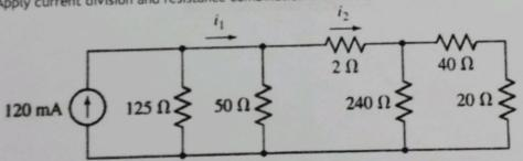
Q.2(b) Examine the current through the  $2\Omega$  resistor by using source transformations. [3] CO1 BL4
